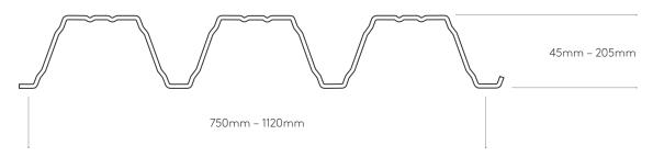
Please note: all Structural Liner Deck profiles can be perforated in the web.
